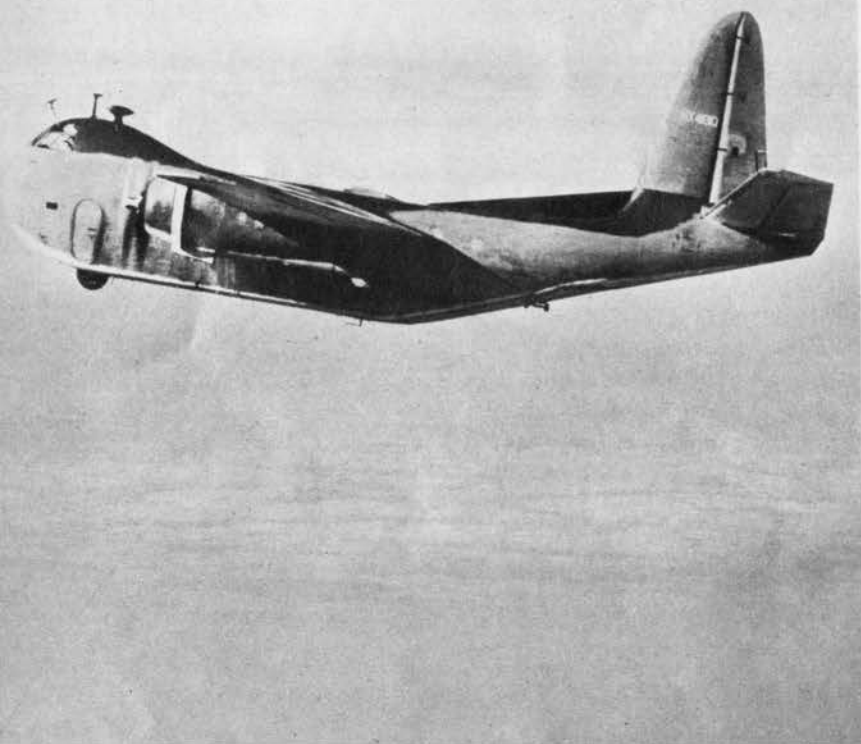
Conestoga has polliwog-shaped fuselage, unique sit in the air. Belly line forms V, with a bulbous head and high tail rising at either end.
